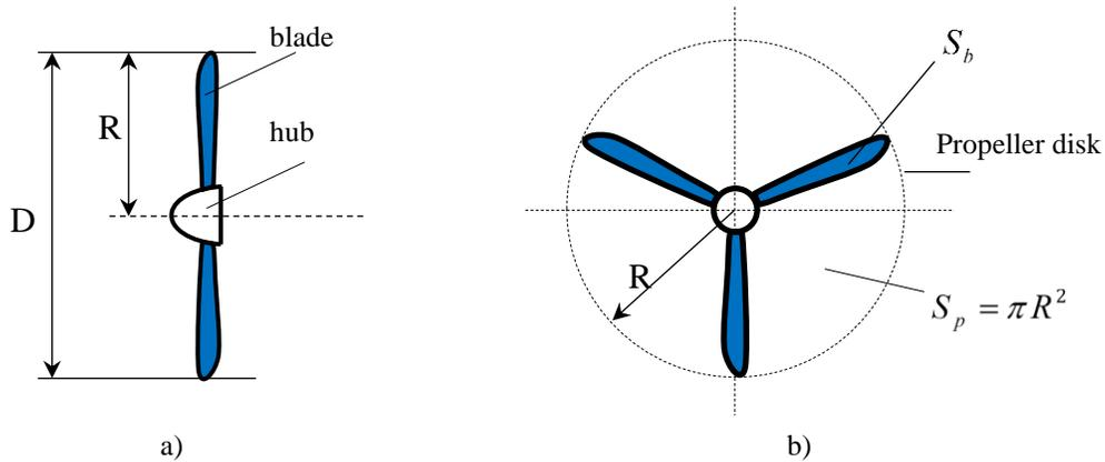
Fig. 10 Propeller geometry: a) lateral view, b) front view
