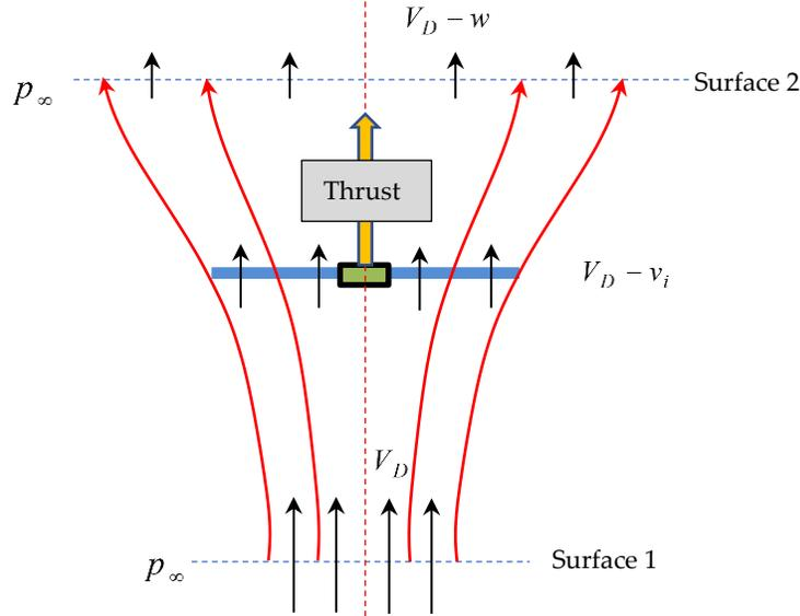
Fig. 19 The stream tube in descent.
