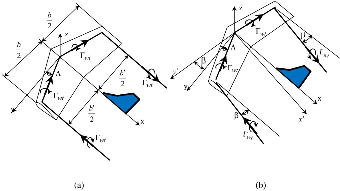
Fig. 1. Model of the wing tip vortex (a) and his effect of the sideslip (b)
