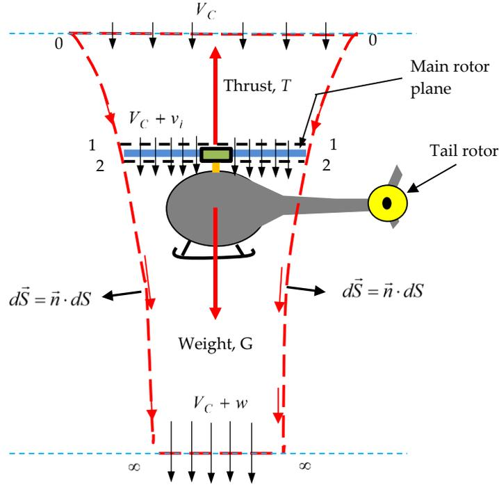
Fig. 18 The axial climbing flight.
