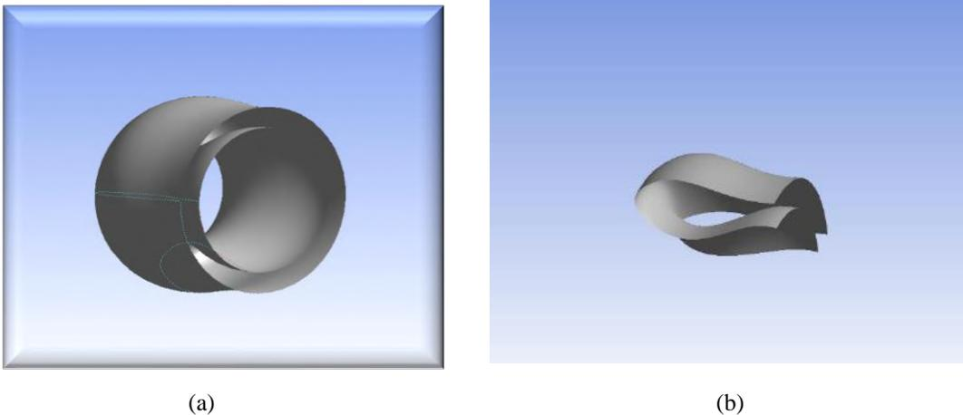
FIG. 31. The 3D view (a) and lateral view (b) of the flame tube
