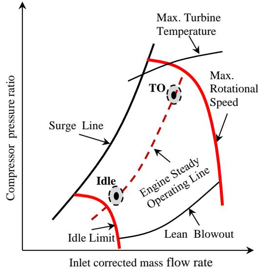
Fig. 28. Engine operating limits on compressor map
