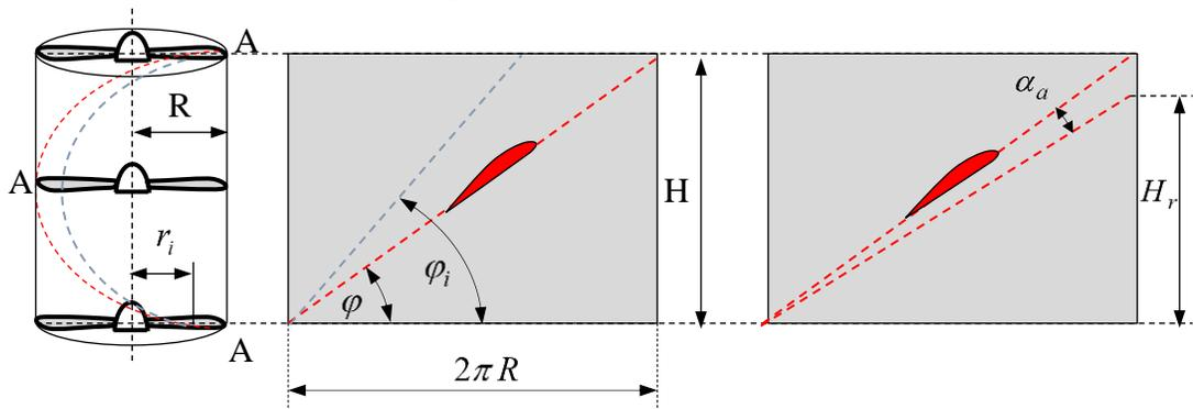
Fig. 11 Theoretical pitch ( $H$ ) and actual pitch ( $H_r$ )
