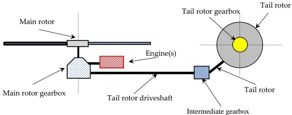
Fig. 16 Typical helicopter constructive model
