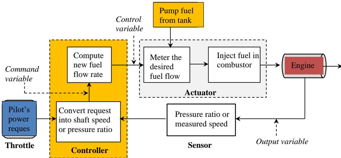
Fig. 26. Engine control system diagram
