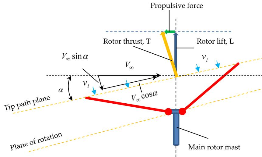
Fig. 20 Rotor in forward flight.
