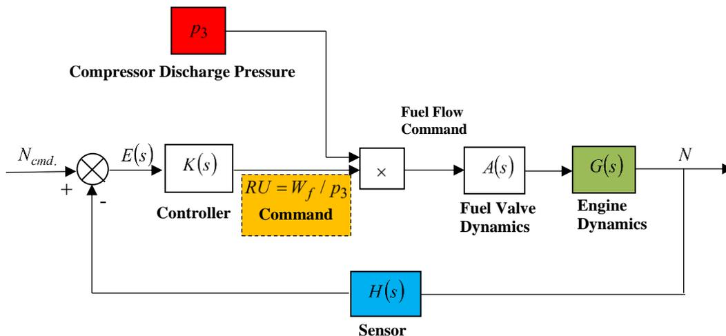
Fig. 27. Controller output to main burner fuel flow rate
