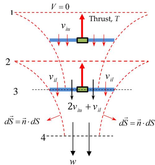
Fig. 22 Control volume for the coaxial rotors
