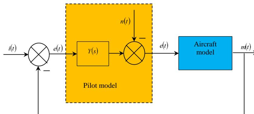
Fig. 24. Linear model of the pilot-aircraft system.
