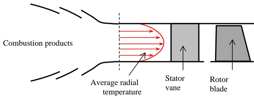
Fig. 29 Turbine blade radial temperature profile
