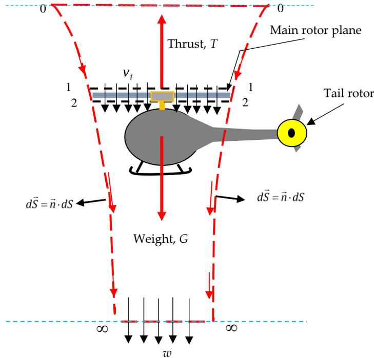
Fig. 17 The main rotor control volume.
