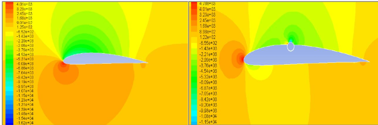
Pressure distribution on the airfoil without cavity
