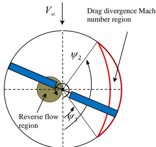
Fig. 5 Helicopter rotor blade
