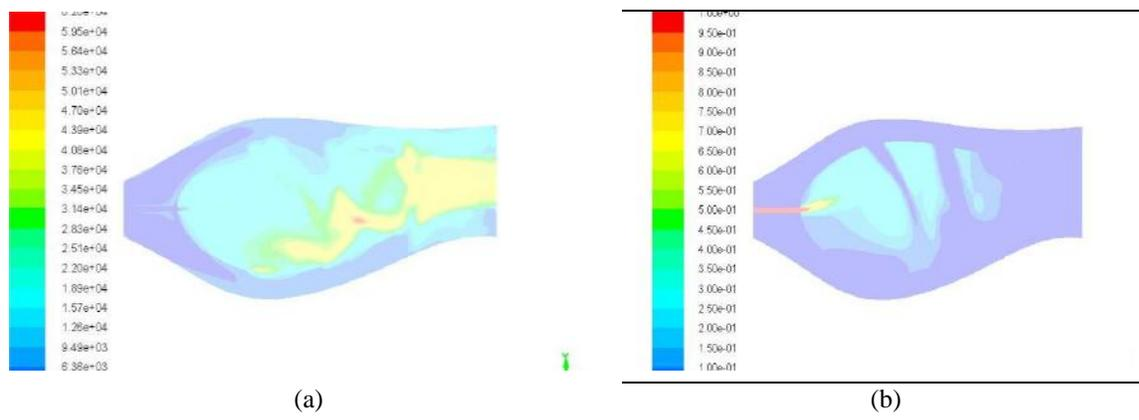
FIG. 36. Turbulent intensity (a) and Mass fraction of jet A fuel (b)
