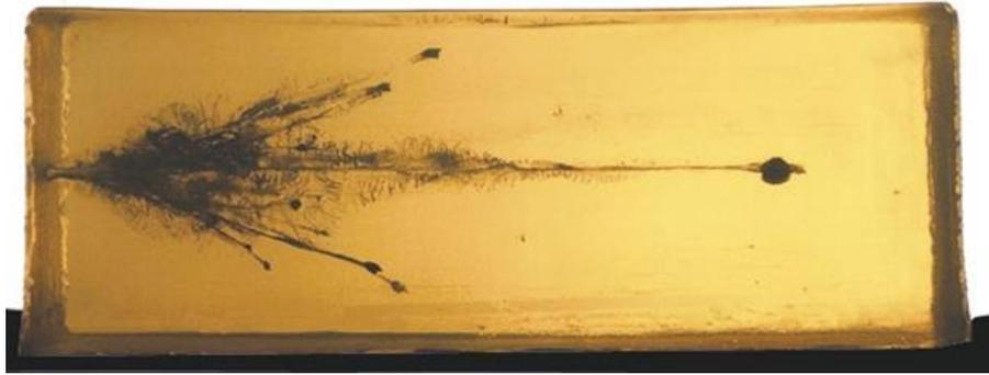
*Figure 2. FAP projectile effect in ballistic gel<sup>[4]</sup>*
