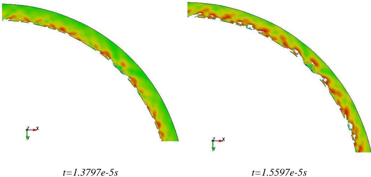
*Figure 4. Strain Fringe LsDyna case 1*
