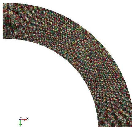
**Figure 6.**  $\frac{1}{4}$  Ring geometry with Weibull distribution of erosion strain
