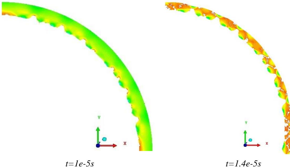
*Figure 15. Strain fringe for Autodyn Weibull distribution case*
