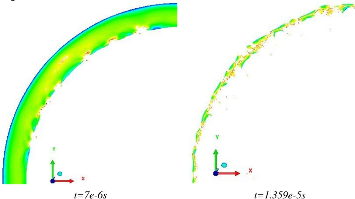
**Figure 13.** Strain fringe for Autodyn Stochastic case
