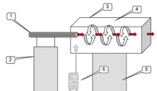
**Figure 2:** Experimental setup: 1. Lab weapon; 2. Weapon support; 3. Frame; 4. LDPE membrane; 5. Support; 6. Specialized sampling pump with glass-fiber filters
