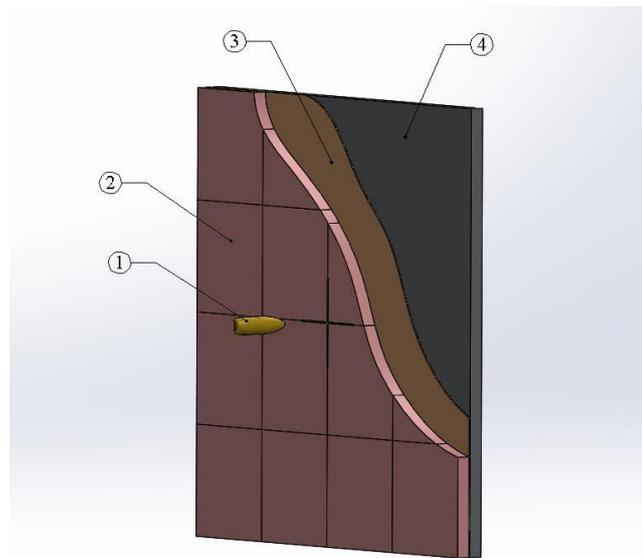
**Figure 1.** *Physical model of the layered structure made of ceramic plates (2), adhesive (3) and high entropy alloy plate (4) at the impact with an armour piercing incendiary tracer 7.62 mm cal. (1)*
