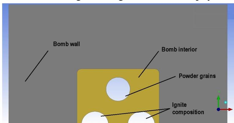
**Figure 1.** The equivalent physical model for a 6/7 powder firing in the manometric bomb
