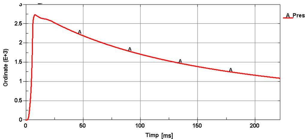
*Figure 4. The pressure versus time graph with data from the manometric bomb*
