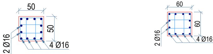
All the stirrups for the columns are  $\text{Ø}10/10\text{cm}$
