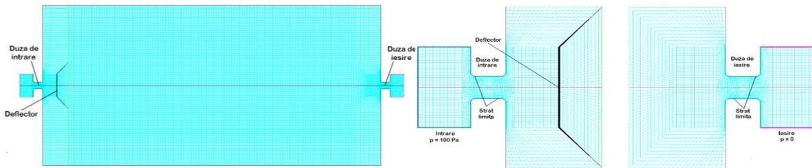
**Figure 1.** a – Axial-symmetric model discretized for the design of the air flow process in the passage compartments – the model with deflector; b – The discretization network in the entry and exit areas from the model.
