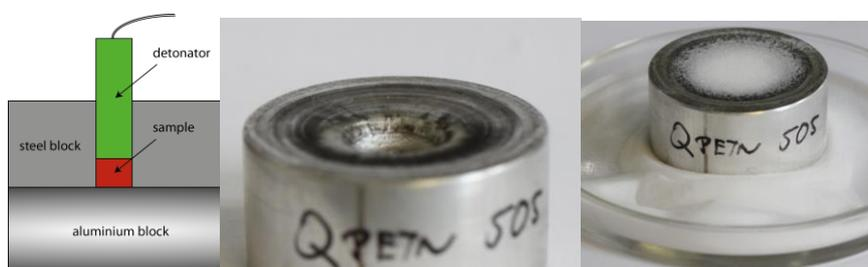
**Figure 3.** Small scale reactivity test SSRT of **2**. a) Schematic set-up b) Aluminum block after the test c) Measuring the volume with sand.
