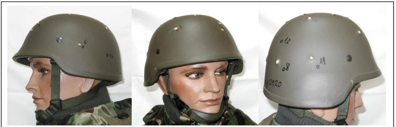
Fig.1. Ballistic limits determination  $V_{BL}$  in accordance with STANAG 2920 and FSP 17grain/1,1 g.
