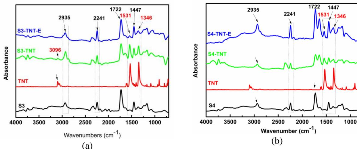
**Figure 4.** FTIR spectra of precursor copolymer powder (S) and membrane of S-TNT and S-TNT-E compared to TNT alone for the S3 (a) and S4 (b) series
