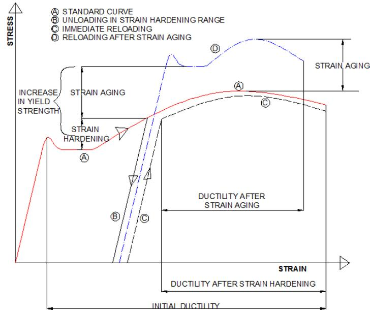
**Figure 3.** Effects of strain hardening and strain aging on stress-strain characteristics of structural steel
