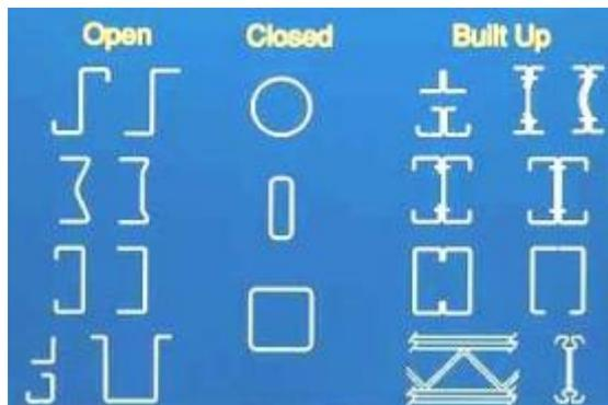
*Figure 1. Cold-formed steel sections*
