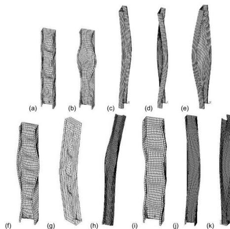
**Figure 2.** *Buckling modes for a C-shape profile in compression*
