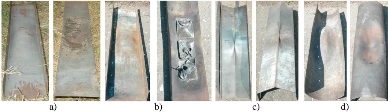
**Figure 4.** Blast wave effects upon: standard plate (a), standard plate with quadrilateral pyramids attached in the center (b), V-shaped plate(c), semi-elliptical shape plate (d)
