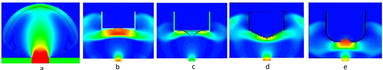
**Figure 6.** Shock wave evolution: formation and propagation of incident wave (a), formation of reflected wave at the interaction with the plate at  $t = 0.07$  ms in the 3D model for: standard plate (b), standard plate with quadrilateral pyramids attached in the center (c), V-shaped plate with  $120^\circ$  peak angle (d), semi-elliptical shape plate (e)
