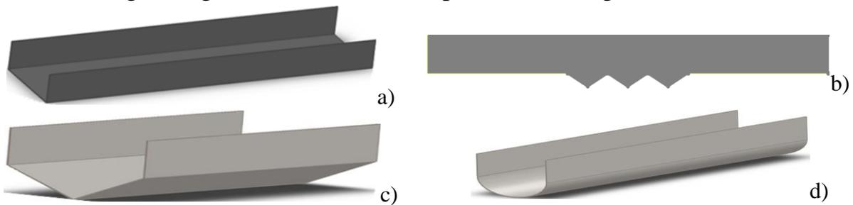
**Figure 1.** Standard plate (a), standard plate with quadrilateral pyramids attached in the center (b), V-shaped plate with 120° peak angle (c), semi-elliptical shape plate (d)
