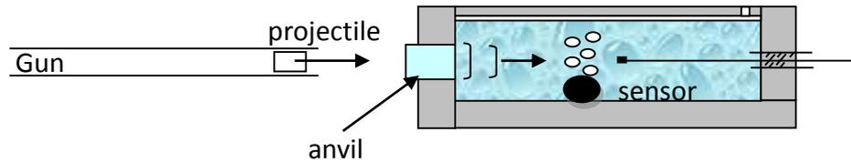
Figure 2: Experimental setup for parametric study of underwater shock wave mitigation by bubble curtain technique.
