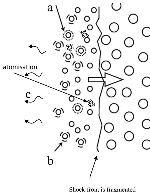
Figure 1: Principle of the underwater shock wave mitigation by bubble curtain. a) Adiabatic compression of bubbles that increase gas temperature and heat exchanges, b) inertial effects that dissipate energy due to viscosity, c) reflected energy by acoustic impedance mismatch, d) loss of energy by bubble atomisation.
