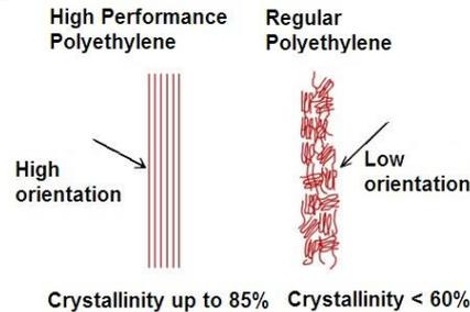
**Figure 1.** Ideal orientation of polymer chains in HPPE and regular PE [4]
