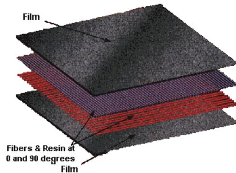
*Figure 2. Spectra Shield structure [7]*
