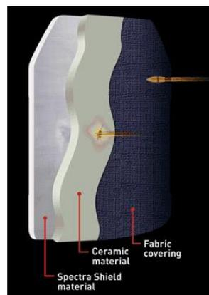
*Figure 5. Configuration of a ballistic protection plate based on ceramic and pressed high-performance polyethylene blocks [14]*
