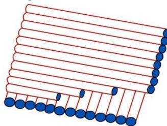
*Figure 4. Construction of Dyneema and Spectra Shield [4]*
